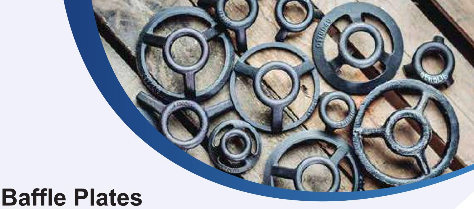
**Drillmax baffle** plates protect float valves, drilling motors, and other bottom hole assembly (BHA) equipment from damage caused by recorders, wireline instruments, or foreign objects dropped down the drill string. Available in spider or ring type.
